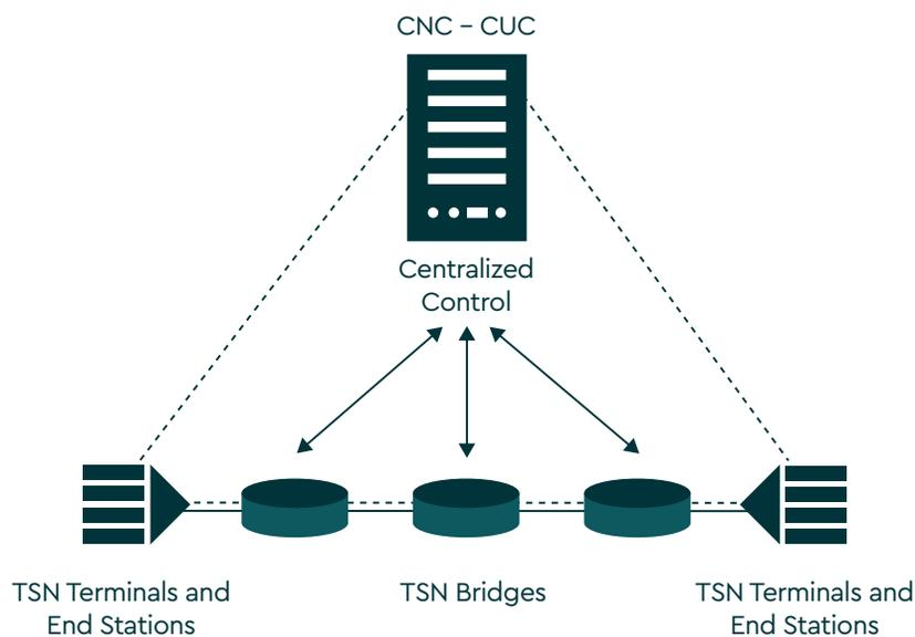
**FIG. 4 Fully centralized model**
