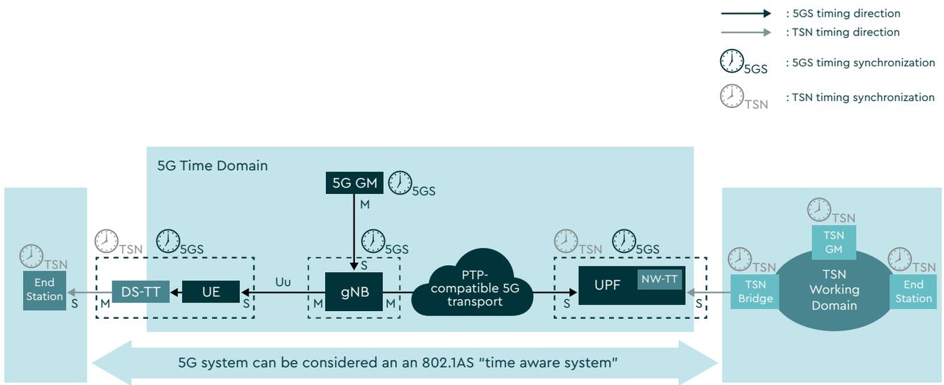
FIG. 2 5G system is modelled as IEEE 802.1AS compliant time aware system for supporting TSN time synchronization
