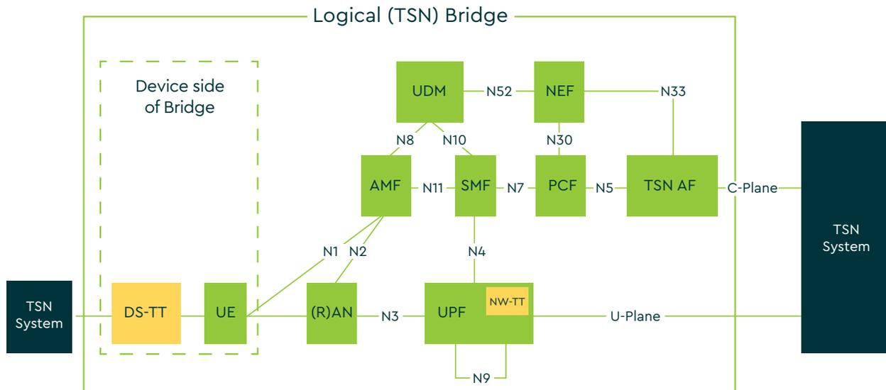
FIG. 1 System architecture view with 5GS appearing as a Time-Sensitive Networking bridge
